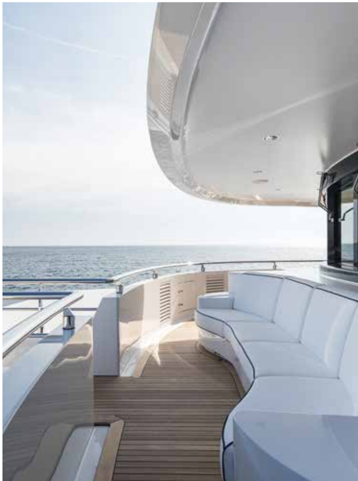
Right and below: wide side deck overhangs and the substantial overhang in front of the wheelhouse, both with a built-in “drip-edge”, are thoughtful standard design touches that will be appreciated in inclement weather
