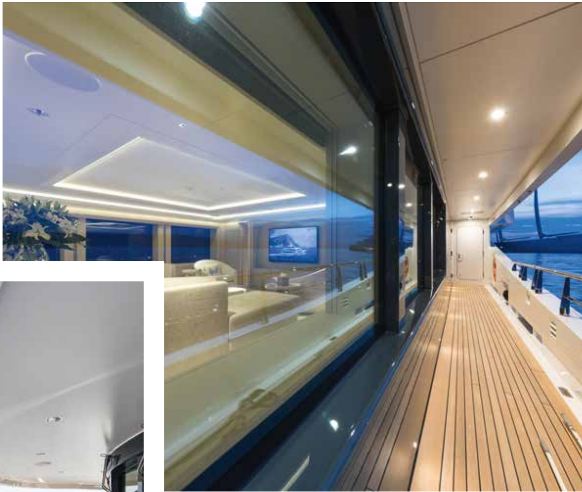
Right and below: wide side deck overhangs and the substantial overhang in front of the wheelhouse, both with a built-in “drip-edge”, are thoughtful standard design touches that will be appreciated in inclement weather
