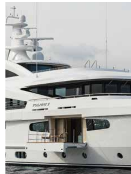
Left: the terrace, on the starboard side of the owner’s suite, deploys in just a few minutes at the touch of a button and the stainless steel and rope railings are stored in a cupboard. As the terrace folds down, a section of teak automatically fills the transition space, creating an unbroken floor for the lounge
